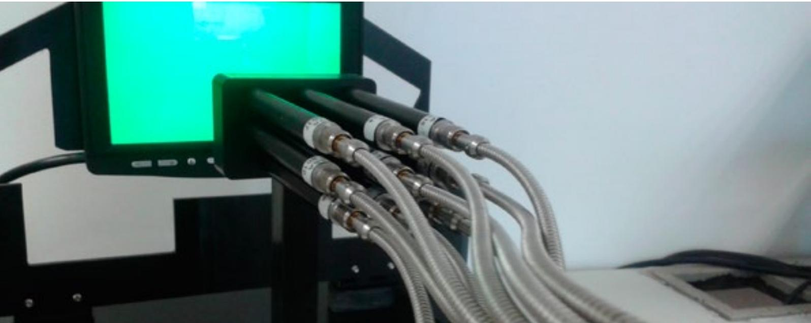
The Feasa Automotive Display Tester is capable of testing the luminance, chromaticity and contrast ratios of automotive displays. The Display Analyser is comprised of detector heads, fiber patch cords and a multichannel sensing module. Up to 10 channels per Display Analyser Module are available for testing. Multiple modules can be 'daisy-chained' together to increase the number of channels.
